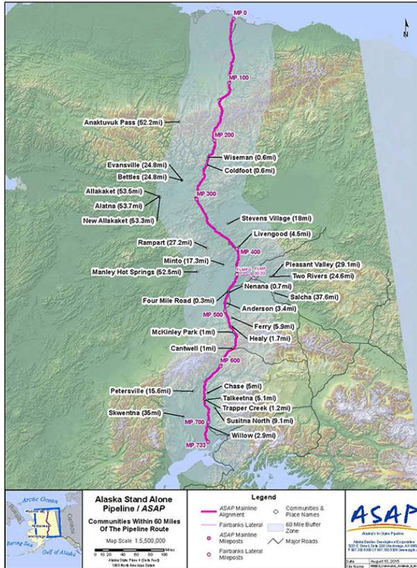
Figure 4. Map of Proposed Alaska Stand Alone Pipeline. The 733-mile low-pressure LNG pipeline would run from Prudhoe Bay to Point Mackenzie, with a 30-mile lateral line between the main pipeline and Fairbanks. Photo: Alaska Gasline Development Corporation (AGDC)
