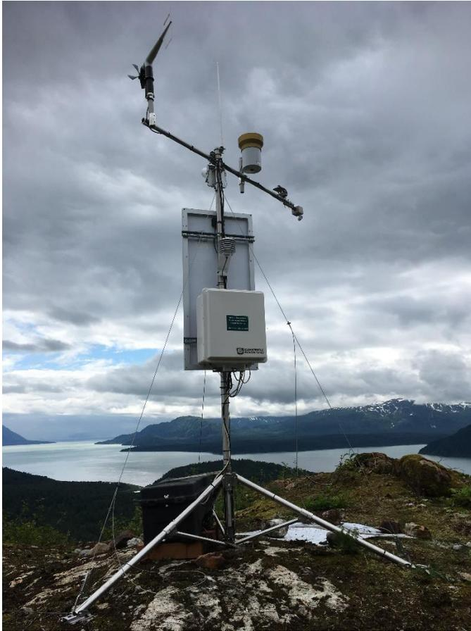
*Figure 2.* Photo of the Nunatak Upper weather station in Glacier Bay National Park. The station at Lone Island is planned to be powered by a fuel cell rather than the solar panel pictured. Sensors may also be positioned closer to the ground to limit visibility. Configuration is otherwise similar.
