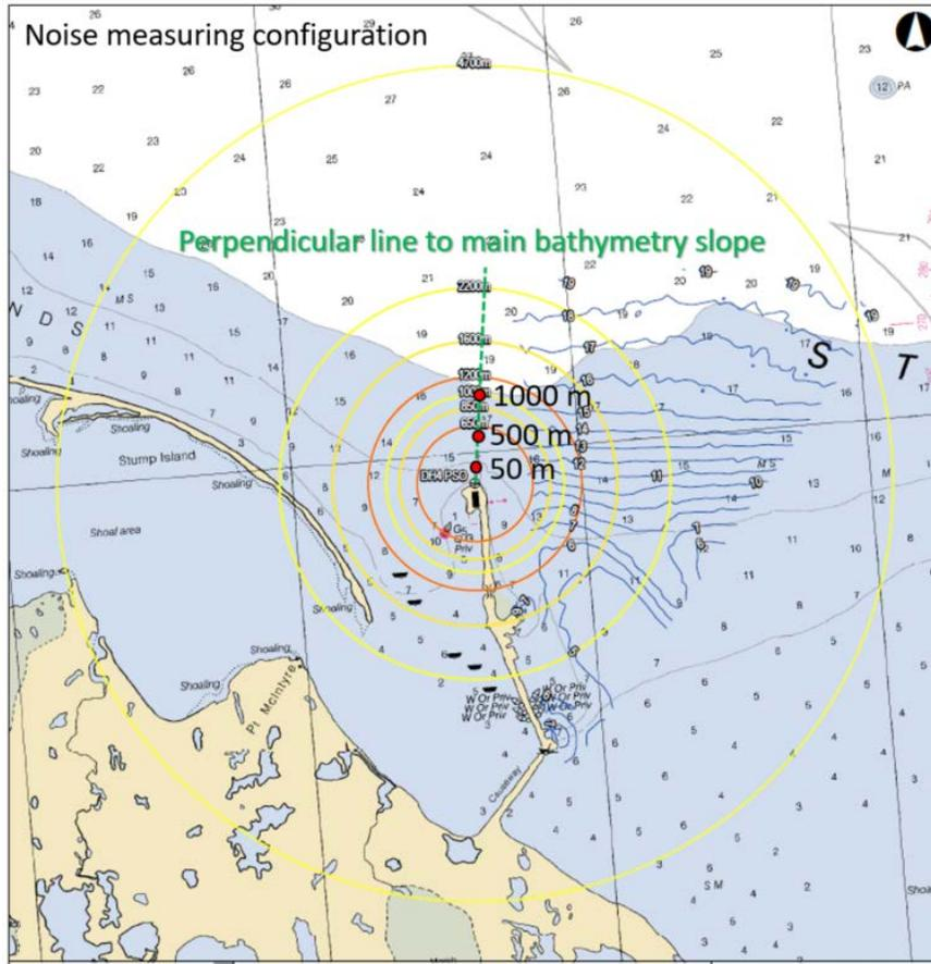
Figure 1: Example of the recommended configuration of the PAM buoys for sound source verification. Three PAM buoys (red dots) would be placed at different distances in line from the pile driver. At least one near-field buoy and one far-field buoy would be required to calculate propagation loss, but a third middle sampling point would increase accuracy.
