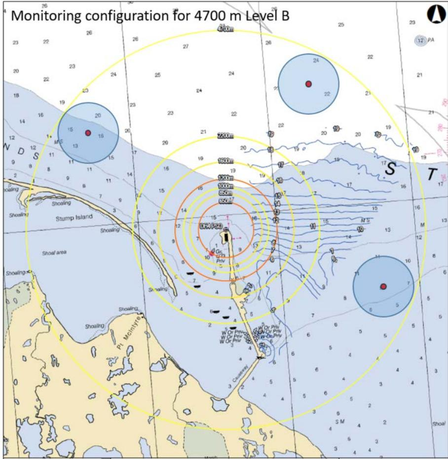
Figure 3. Example of monitoring configuration for real-time PAM. Three moorings (red dots) placed at equidistant intervals from each other with their respective detection ranges of 860 m (blue areas) corresponding to their distance to the edge of the 4,700 m monitoring zone.
