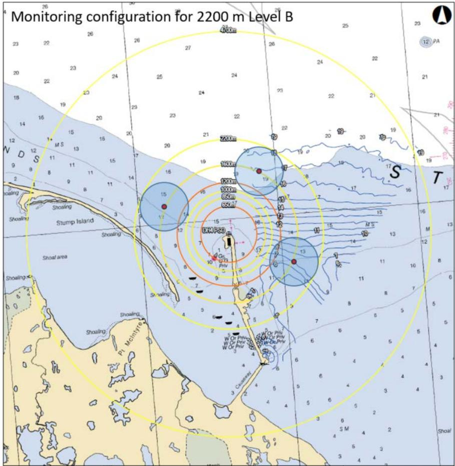
Figure 2. Example of monitoring configuration for real-time PAM. Three moorings (red dots) placed at equidistant intervals from each other with their respective detection ranges of 860 m (blue areas) corresponding to their distance to the edge of the 4,700 m monitoring zone.
