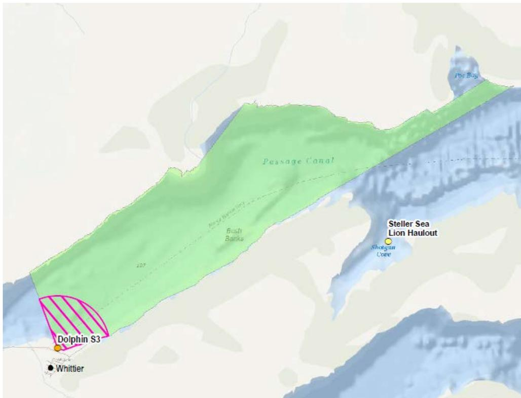
**Figure 3. Project location with AKDOT&PF proposed monitoring zones. The light green is the vibratory hammering monitoring zone extending 12 km, and the hatched is the impact monitoring zone that extends 1.2 km.**
